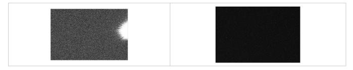
Download a sample unprocessed dark frame taken with the OGMA AP26CC camera at room temperature.
