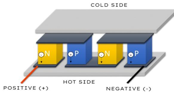
The TEC system is controlled by a PID algorithm, which allows the TEC to be precisely regulated towards the target temperature with 0.1°C deviation. Such efficient cooling system guarantees the stability of ultra-low noise mode and quality of the camera image.
