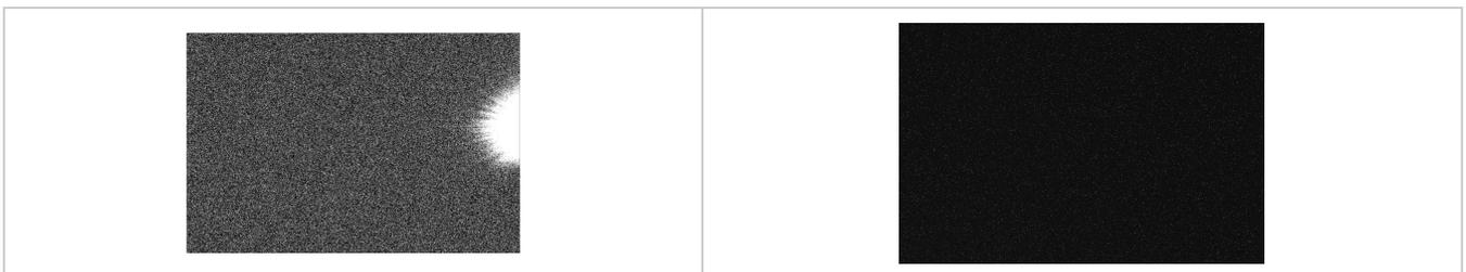
[Download a sample unprocessed dark frame](#) taken with the OGMA AP26CC camera at room temperature.
