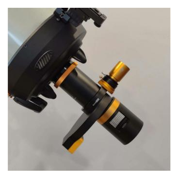
Most cooled cameras have six tapped holes on the front plate around the opening of the imaging sensor. The six holes are distributed around a circumference of 62mm in diameter.
